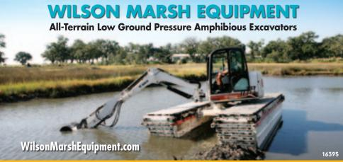
These machines are great for pipeline laying, right of way clearing, land reclamation, levee building, disaster rescue & clean up, power line construction and any work in soft terrain. Attachments include bush cutters, vibrator pile drivers, augers, buckets, saws and much more.
