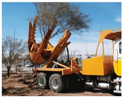
The spoon shaped blades on a Big John Transplanter are inserted into the ground along a curvilinear track forming a totally enclosed pod of roots and soil. The tree is then removed from the soil and transported to its new home.
