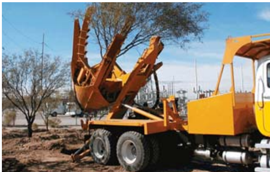
The spoon shaped blades on a Big John Transplanter are inserted into the ground along a curvilinear track forming a totally enclosed pod of roots and soil. The tree is then removed from the soil and transported to its new home.
